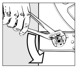
■ Using a pipe wrench turn the lefthand transit bar 90°.
